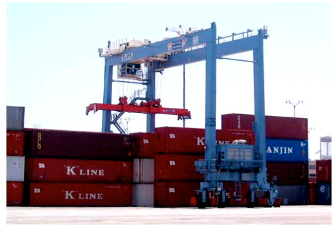
Figure 1 Typical Rubber Tired Gantry (RTG) Crane
